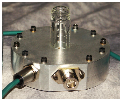
Reaction Cavity and Infrared Thermometer with 5.0 ml Wheaton(tm) Reaction Vial
