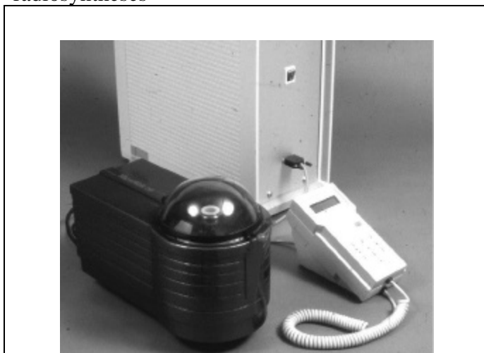
Figure 2C. Series-produced cavities (MicroWell 10) based on the concepts in Figure 2A and 2B have been used in a number of PET-related procedures (see Table) (Labwell AB, Uppsala, Sweden)
